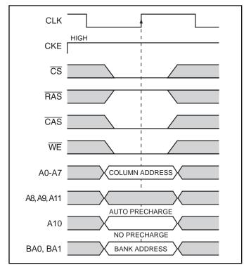
The starting column and bank addresses are provided with the WRITE command, and auto precharge is either enabled or disabled for that access. If auto precharge is enabled, the row being accessed is precharged at the completion of the burst. For the generic WRITE commands used in the following illustrations, auto precharge is disabled.
